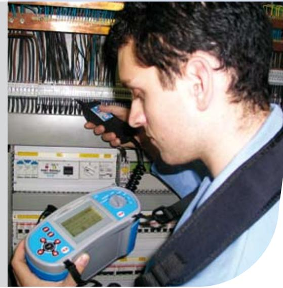
EurotestLITE is a complete multifunction installation safety tester with integrated memory module. Lightweight instrument is ergonomically designed and offers the customer one of the best price-performance ratio on the market. Windows compatible PC Software Eurolink enables downloading of the test data and creation of test reports.
